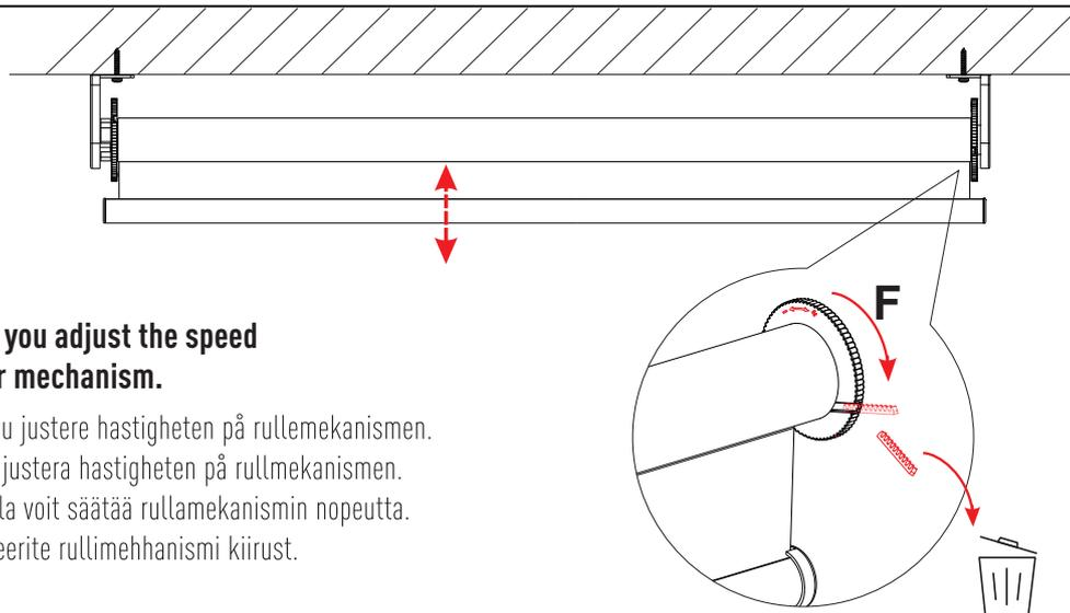
This is how you adjust the speed of the roller mechanism.
